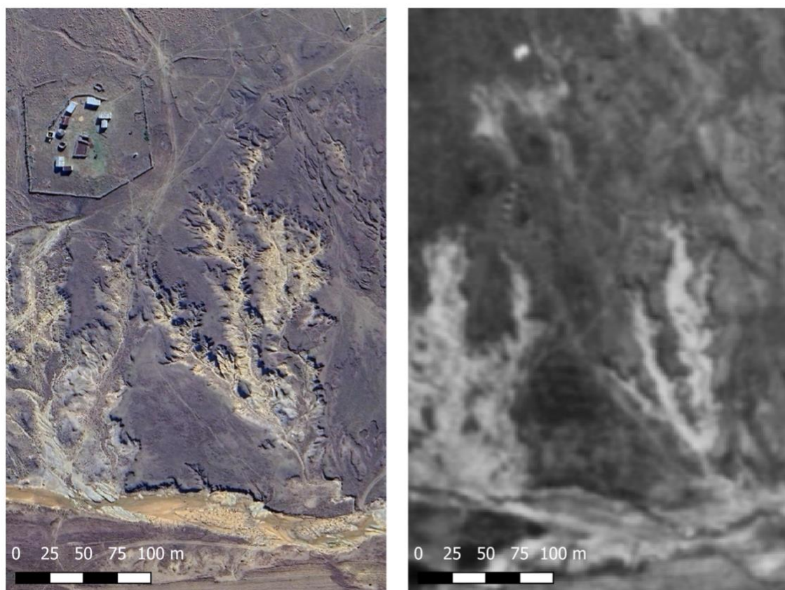
Figure 10. Extension of a dendritic donga at Magongoloza River identified from recent satellite imagery (left) (Google Maps/Airbus/Maxar) and a historical orthophoto from 1944 (right) (National Geo-spatial Information [NGI]).
