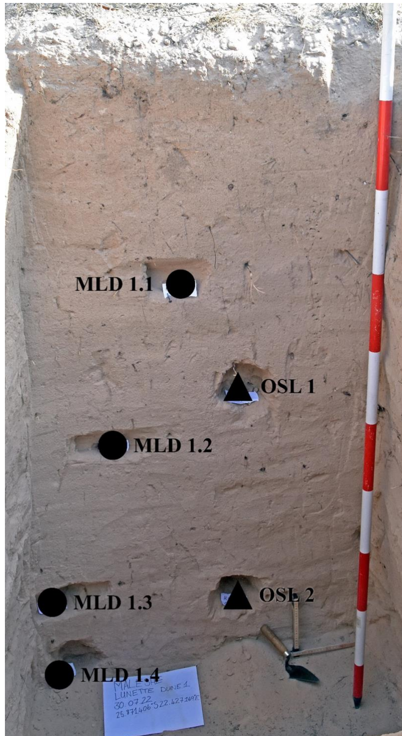
Figure 3. Photograph of geotrench MLD 1 located on the inner dune associated with Maleshe Pan. Bulk sediment sampling locations are marked with circles, while the triangles denote OSL sampling locations. Sample IDs correspond with bed names. Each pole section=25 cm.
