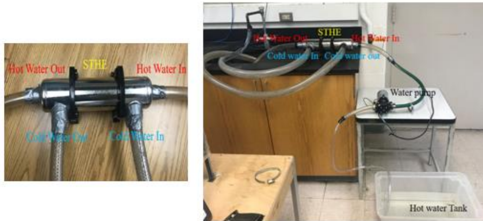
Figure 1. Schematic Diagram and Experimental Setup of STHE Prototype
