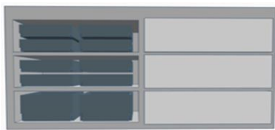
Figure 4: 3D Model of Mobile Cooling System with Two Sections and Six Chambers
