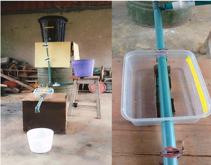
Plate 1.4: An image of the magnetized water production unit's magnetic treatment setup
